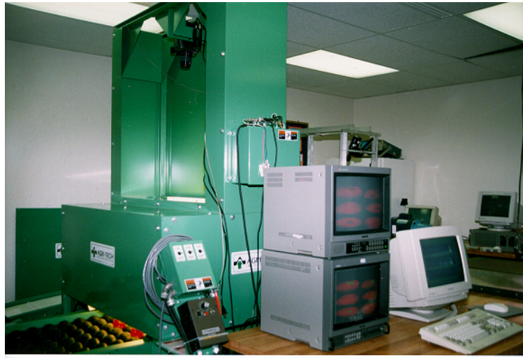
Figure 7. A snapshot of NIR machine vision system for apple quality inspection and stem-end/calyx identification
